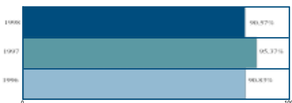
Figure 15: Water Supply Zones Complying with pH Standard
